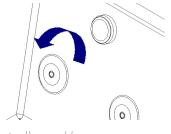
To do that, unscrew the jet cover anticlockwise. Now clean the cover, the inlet aperture and the outlet aperture thoroughly.
